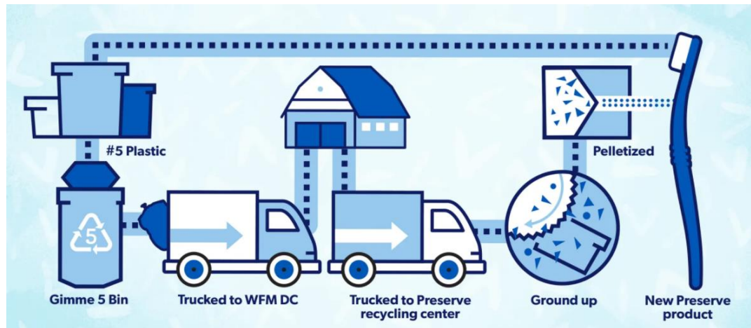
FIGURE 14 HOW THE PRESERVE PLASTICS WORK [33]
